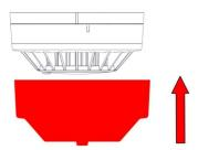
During site works place the plastic cover to the detector (only for BSR-6155/A & BSR-6157/A) as shown in the picture above to protect the device from dust.
