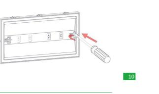
Attention!! The 6 plastic latches (A) must be secured (click sound). This requirement is important to ensure the IP65 rating. Power on the
