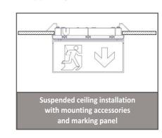
After finishing the installation you must power the luminaire for at least 24 hours in order to completely charge the battery. The rated autonomy duration can be achieved after that time.
