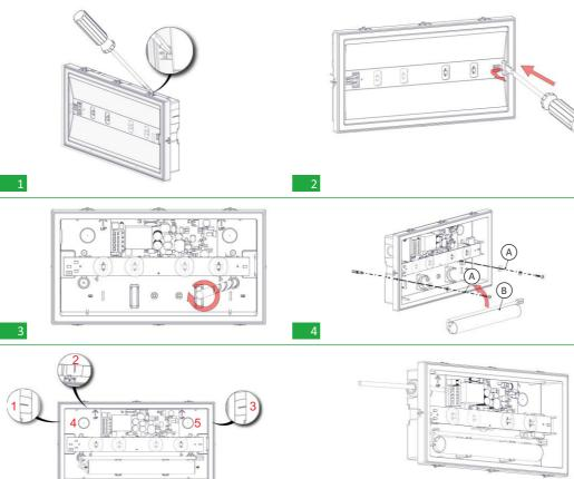
Drill one of the available 5 holes with a 16-18mm drill bit. Install the included rubber gasket and pass through the power cables. Install the included tie (if needed) to fasten and securely the power cables.
