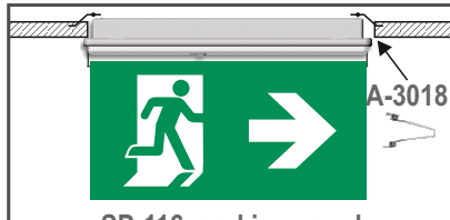
SP-116 marking panel Suspended ceiling installation with A-3018 mounting springs and SP-116 marking panel
