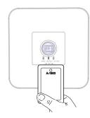
Test and Faults Reset operations with the A-1900 card (not included and available after request). For lights test, you must place the card in front of the TEST indicator and remove it immediately. For Autonomy Test, you must place the card in front of TEST and hold it for 5 to 10
