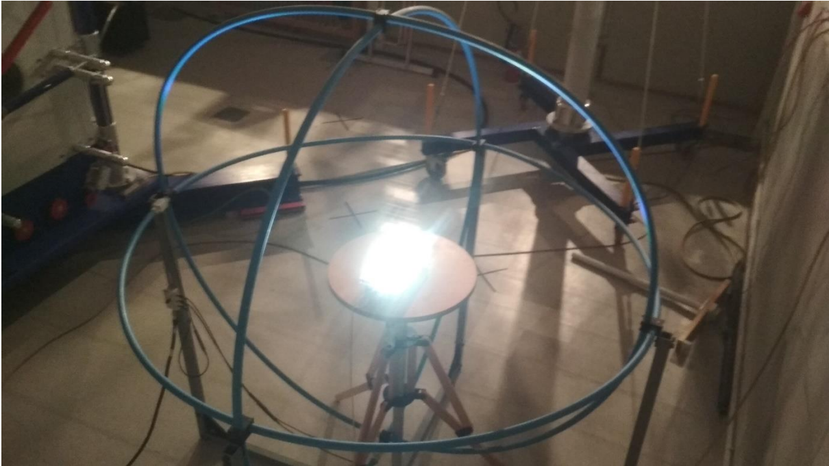
Photo 9.1: Setup for radiated magnetic emissions test (9kHz-30MHz)
