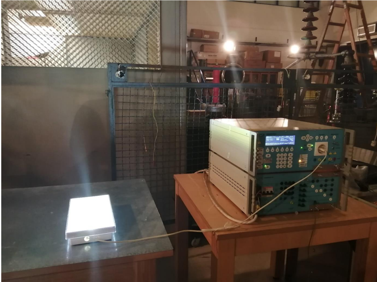
Photo 18.1: Setup for voltage dips and short interruptions test
