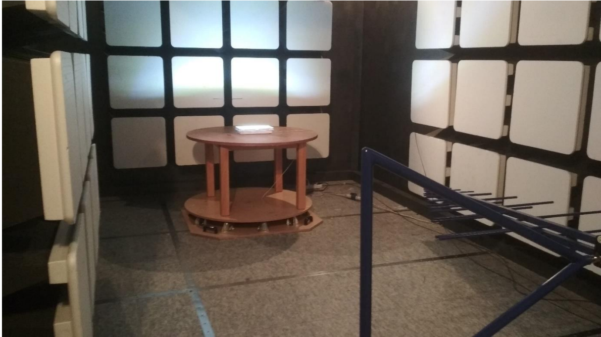
Photo 8.1: Setup for radiated emissions test
