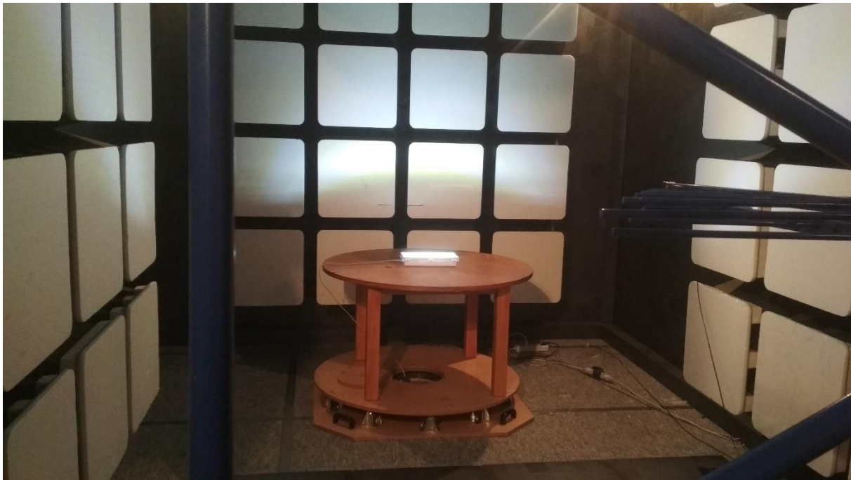
Photo 13.1: Setup for RF electromagnetic field test
