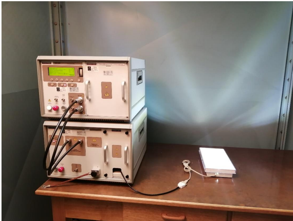
Photo 15.1: Setup for surge test
