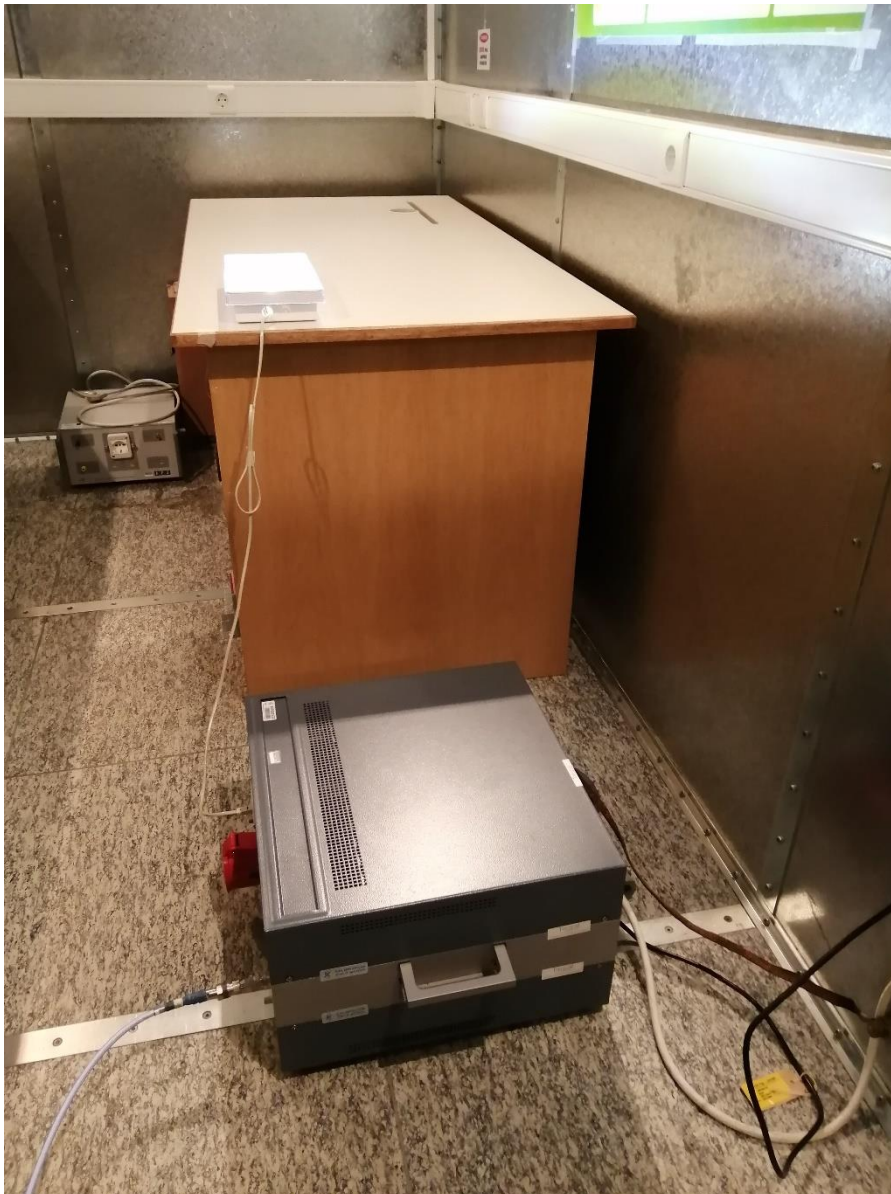
Photo 8.1: Setup for conducted emissions test
