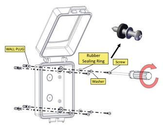
Place the box on the wall and fasten it with the supplied mounting accessories. WARNING!!! The lid should be fitted.
