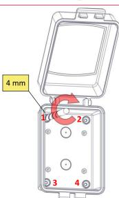
Drill the four available holes with a 4mm drill to mount the box on the wall.
