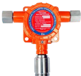
TC100N Ex d IIC T6 Gb, -20°C ≤ Ta ≤ +60°C
