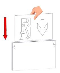
**Step 1:** Install the required pictogram. There is one blind pictogram for one-sided marking.
