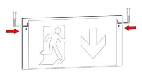
Step 2: Place the holding accessories to the marking panel.
