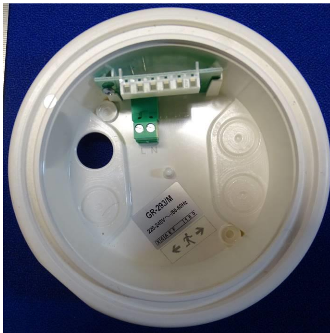
Luminaire Interior (Main Enclosure)
