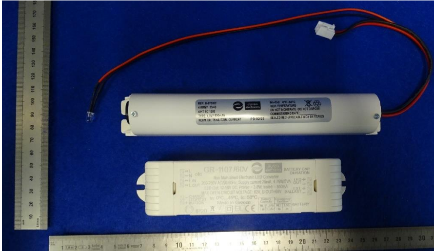
Controlgear GR-1107/60V with battery
