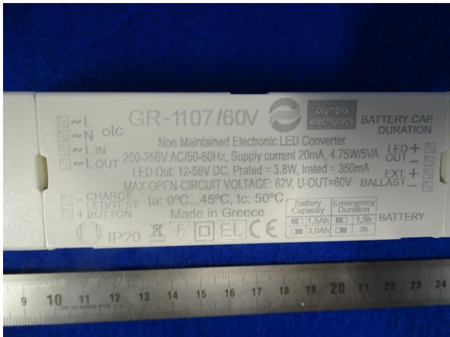
Controlgear GR-1107/60V markings
