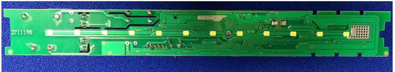
Control gear secondary side / light source
