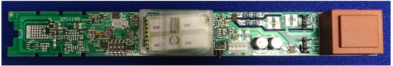
Control gear primary side
