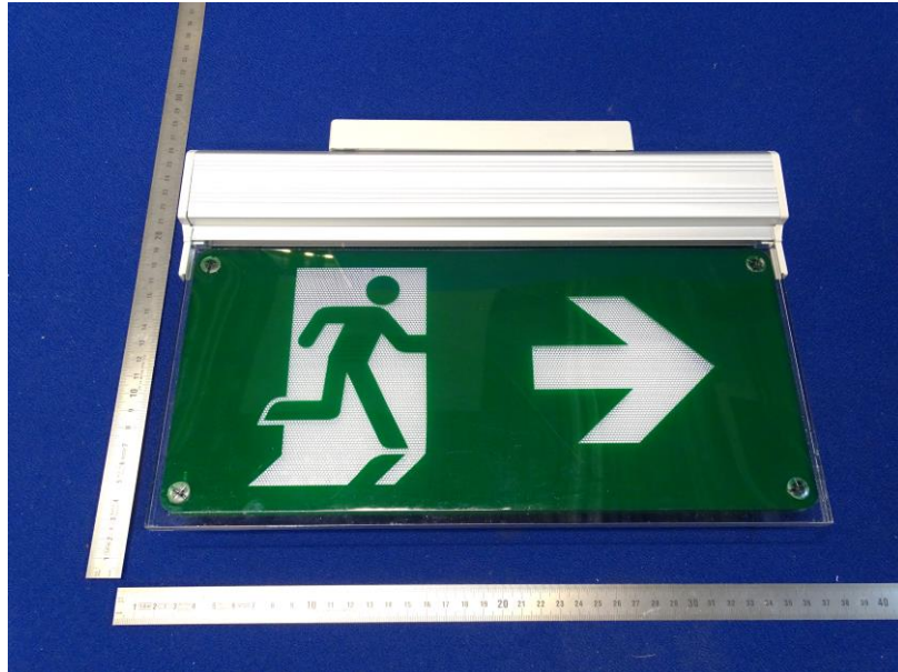
Photograph 1: Luminaire Overview – Emergency Exit Luminaire Model No. ZLD-34/24V/ADR/EM (Front)
