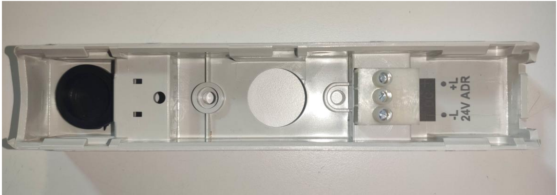
Photograph 7: Means of Connections (Terminal)
