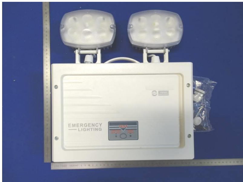
Photograph 1: Luminaire Overview – Two spot emergency luminaire Model No. GRL-37/180/WP/ADR (Front)
