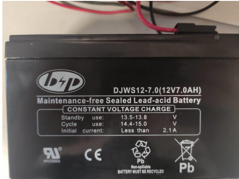
Photograph 11: Built-in rechargeable battery
