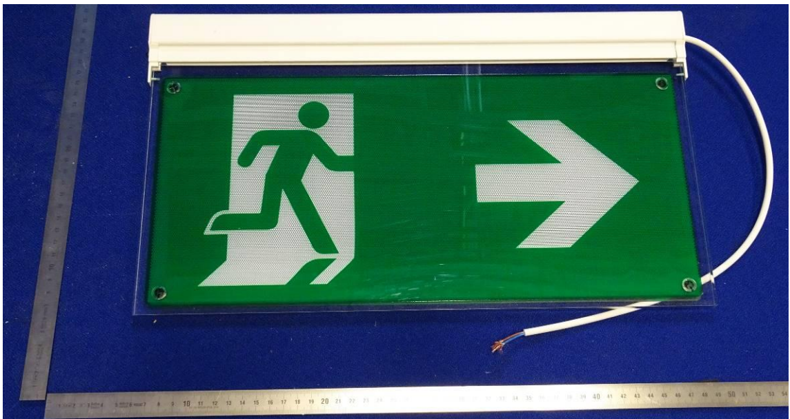
Photograph 2: Luminaire Overview – Emergency Exit Safety Sign Model No. MLD-44D/w (Rear)
