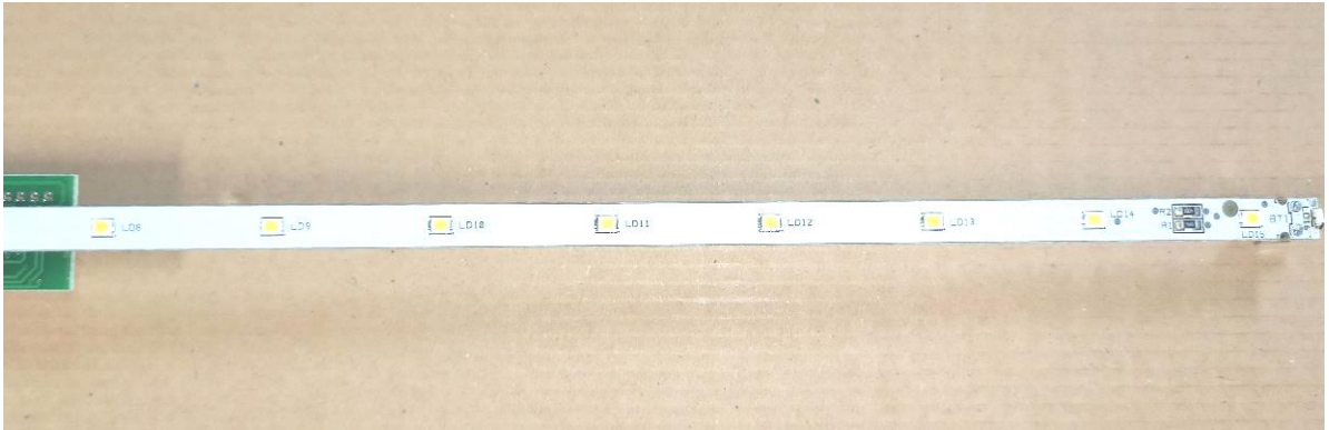
Photograph 7: Built-in LED module
