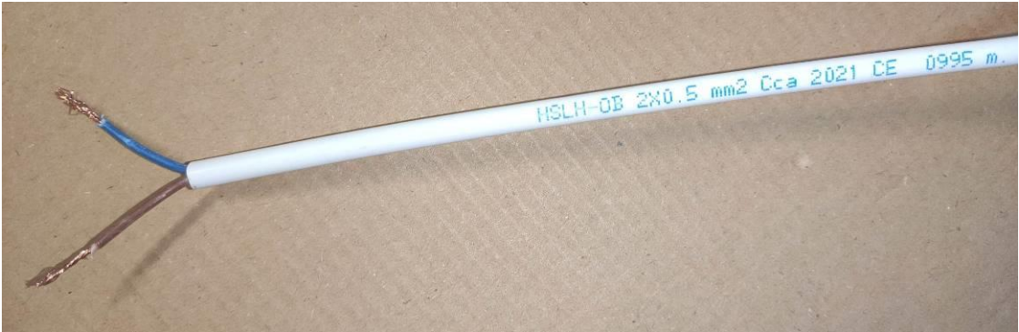
Photograph 9: Means of Connections (Connecting Leads (Tails))
