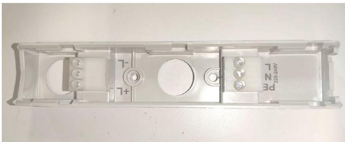
Photograph 10: Means of Connections (Terminal)
