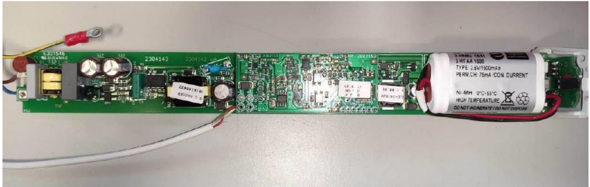
Photograph 5: Built-in lamp controlgear (Top)
