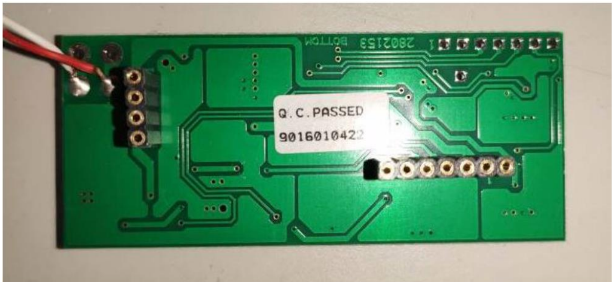
Photograph 8: Built-in LED module
