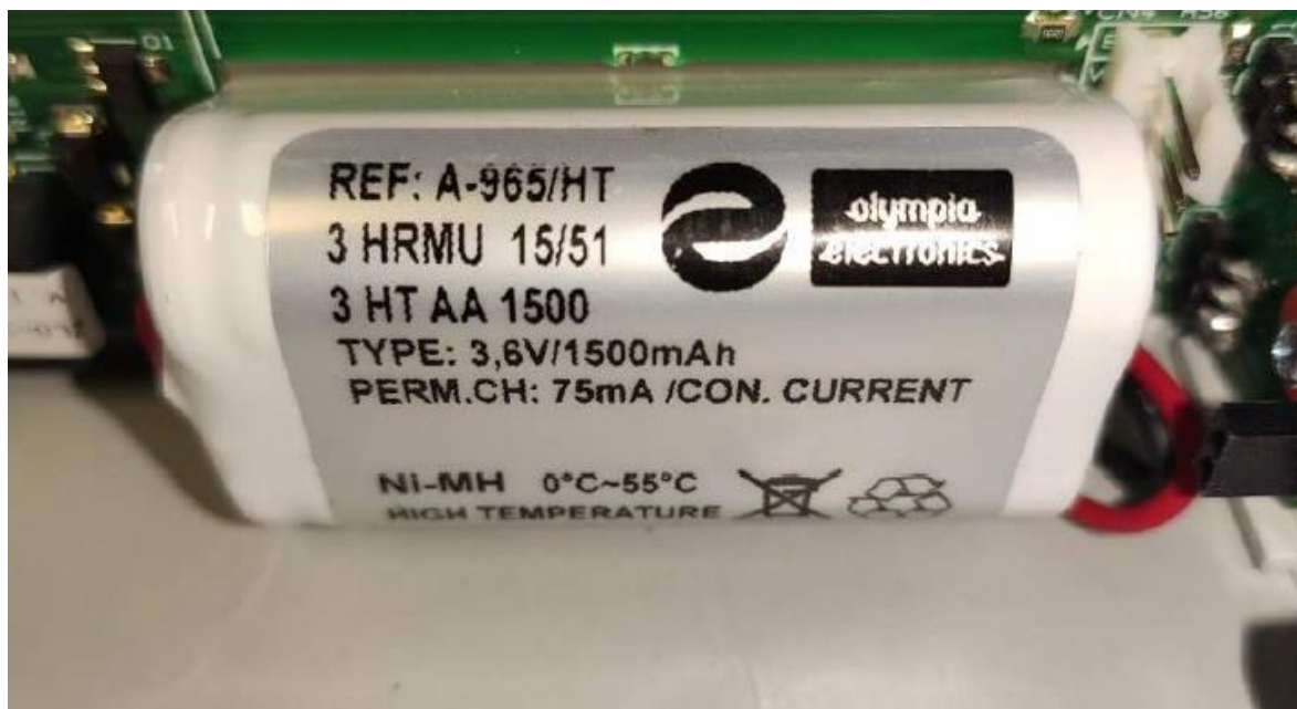
Photograph 9: Built-in rechargeable battery
